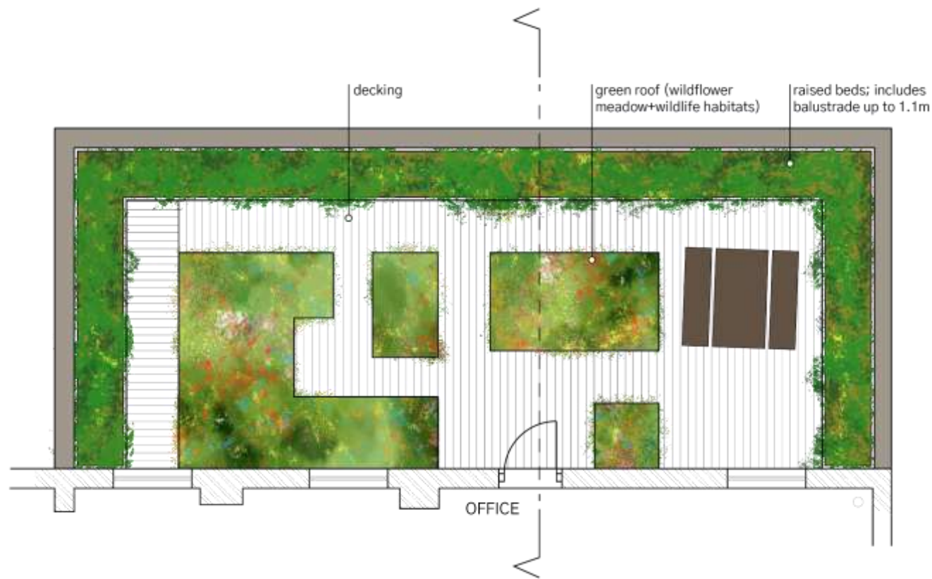
Boiler House Green Roof. Client: Sow the City
